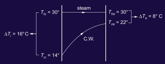
$$\therefore \qquad \text{(LMTD) of } HE = \frac{\Delta T_i - \Delta T_e}{\ln \frac{\Delta T_i}{\Delta T_e}} = \frac{16 - 8}{\ln \left(\frac{16}{8}\right)} = 11.54^{\circ} \text{ C}$$
