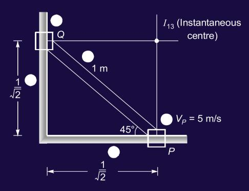
Treating like the elliptical trammeds. Rod motion (P, Q) (By sitting on  $I_{13}$ )
