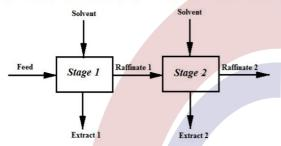
Components B and C are immiscible. 60% of A in the feed is extracted in *Stage 1*. The equilibrium relation is given by  $Y^* = 1.5 X$  where. X = moles of A per mole of B in raffinate
