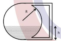
The estimate of liquid height (in m) to store V = 30 m<sup>3</sup> of water in R = 3 m tank, after performing ONE iteration of Secant method, using 1 m and 3 m as two initial guesses of \_\_ (rounded off to second decimal place).
